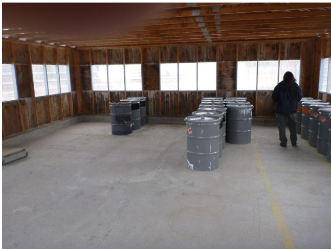
A good example of container management in a STSA, with at least 2 feet of aisle space in between rows and visible waste labels.
