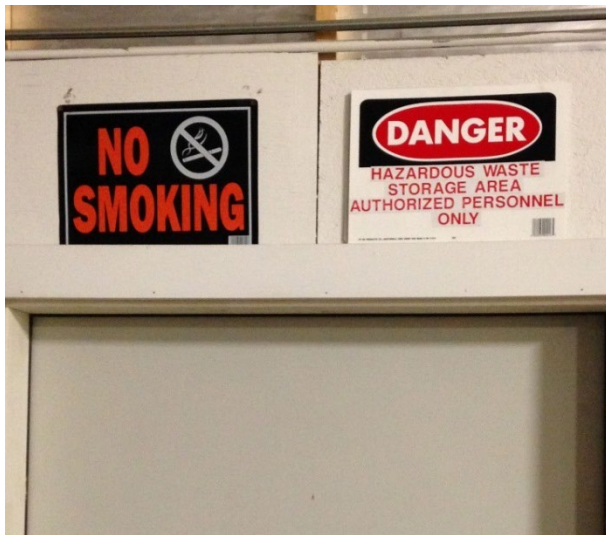
Correct signage at the entrance to a short-term hazardous waste storage area where ignitable waste is stored
