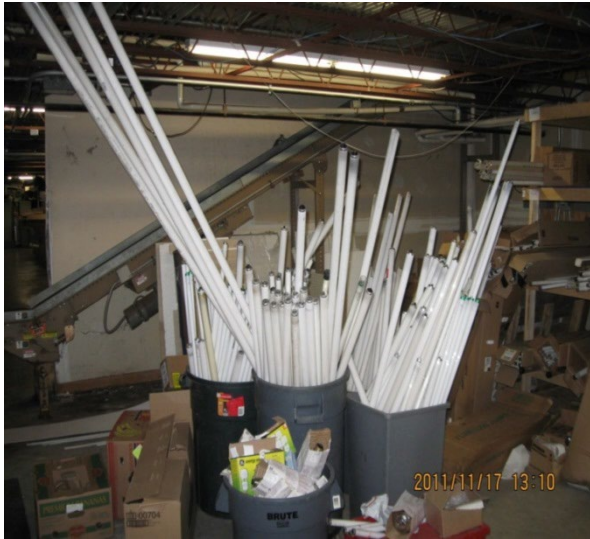
Improper storage of waste lamps – lamps are not packaged in containers adequate to prevent breakage
